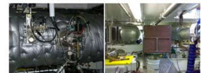
Figure 3.4: Urea injection and PM filter burner.
