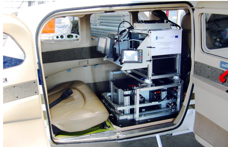
LiteMapper 6800i LiDAR system installed inside the plane
