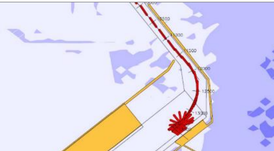
SHIPMA simulation of arrival of 150,000 DWT bulk carrier under moderate conditions at Khalifa Port, Abu Dhabi UAE (CH2M Halcrow)
